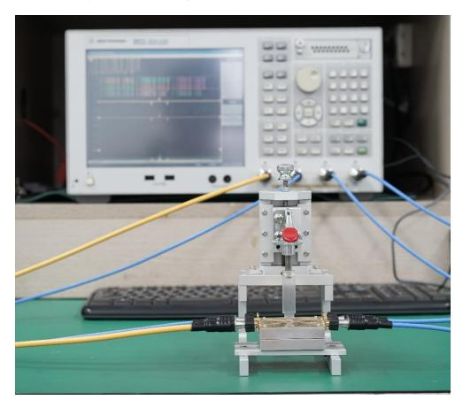
Figure 5. Test Setting to Measure the CMX09E03 S-parameters
