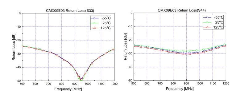
Figure 3. Test Plots of Return Loss (-55 °C, 25 °C, and 125 °C)
