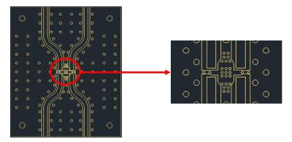
Figure 9. Cleaning the PCB Surface Where the CMX09E03 is Soldered
