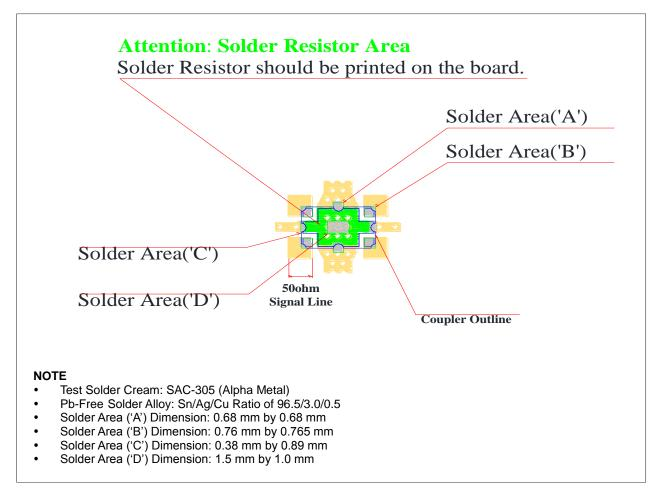
Figure 8. Recommended PCB Layout and Solder Mask Pattern
