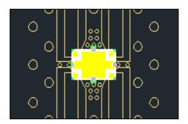
Figure 11. Placing the CMX09E03 on the 9 Points of the PCB Surface
