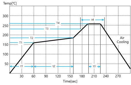
Figure 12. Thermal Reflow Profile
