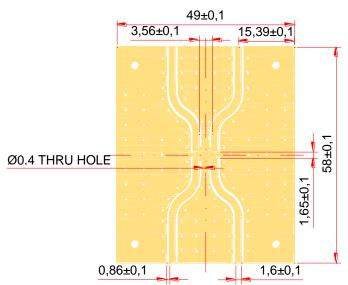
Figure 6. RN2 Test Board Layout
