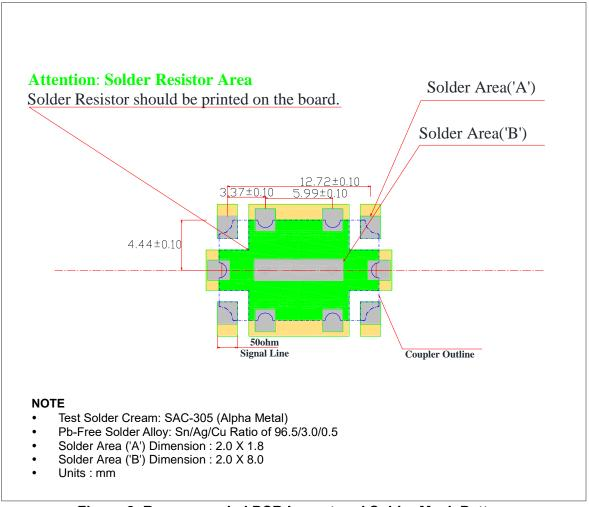
Figure 8. Recommended PCB Layout and Solder Mask Pattern
