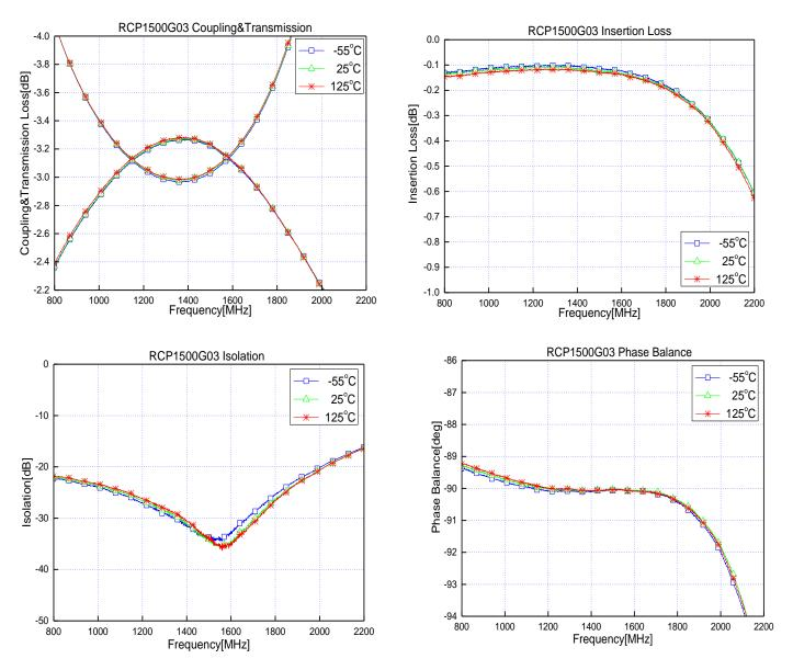
Figure 4. Test Plots of Coupling and Transmission Loss, Insertion Loss, Isolation, and Phase Balance (at -55 °C, 25 °C, and 125 °C)
