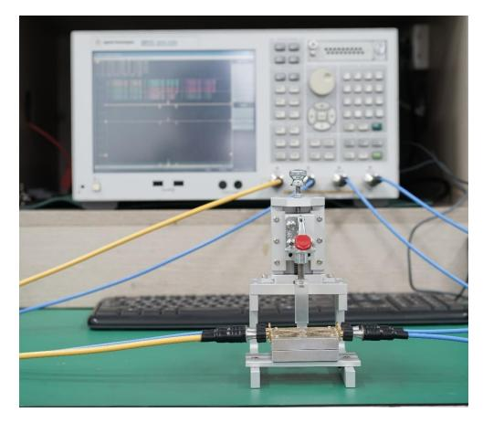
Figure 5. Test Setting to Measure the RCP1500G03 S-parameters
