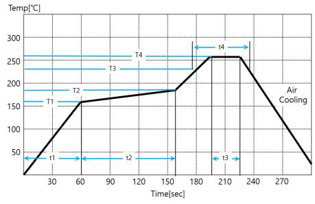
Figure 12. Thermal Reflow Profile
