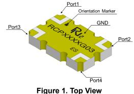
RCP1500G03 port configurations in table1 depending on how input signals are split. The Case 1, Case 2, Case 3, and Case 4 configurations mean that one input signal is split into two output signals. When port 1 is defined, the other ports are defined automatically.
